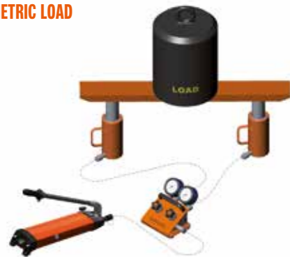
Recommended total cylinder capacity = 1.5 x load
