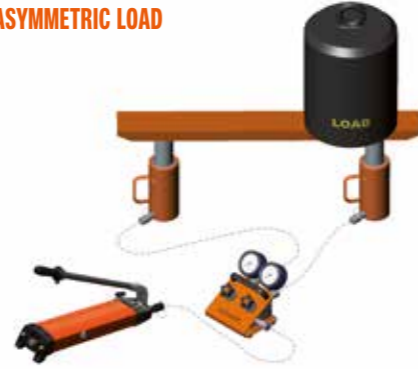
Recommended total cylinder capacity = 2 x load
